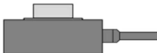
FIG.4 The load is applied to the center of the moving surface
