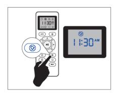
Press button on Remote Control, and then the hour section begins to flash in the Cleaning Schedule display setting window.
