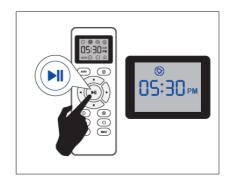
And then press the button, the Robot will "BEEP" when the Cleaning Schedule setting completed.
