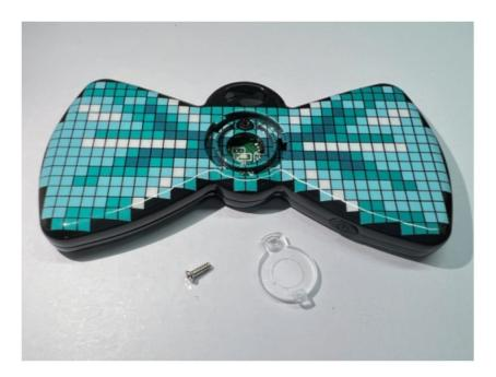
Open the Bluetooth tracker and remove the battery.
