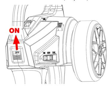
• CONNECT THE BATTERY TO THE ESC SWITCH ON THE ESC
