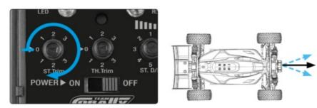
The steering trim is used to adjust the steering setting so that the car moves in a straight line without using the steering wheel to compensate.
