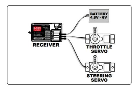
Install the Receiver in your model using double-sided Velcro. Velcro will hold the receiver in place and protect it from vibrations. Mount the antenna up and away from the vehicle in an antenna tube. The higher up the antenna is, the better signal it will receive.
