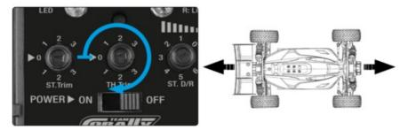
The throttle trim is used to adjust the setting of the neutral position of the throttle without using the throttle/brake trigger to compensate.
