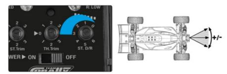
Use this function to adjust the steering travel of your model. If the model understeers while cornering, add steering by turning CW of the D/R button. When the model oversteers, take away steering by turning CCW of the D/R button.
