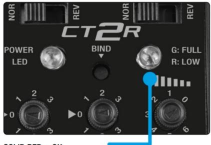
SOLID RED = OK FLASHING RED = Low Voltage (Replace batteries)
