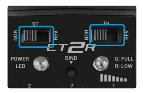
**ST.REV** (**Steering Reverse**): This function reverses the rotation direction of the STEERING servo. **TH.REV** (**Throttle Reverse**): This function reverses the rotation direction of the THROTTLE servo.
