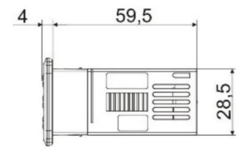
Instrument XR60CHC shall be mounted on vertical panel, in a 29×71 mm hole, and fixed using the special bracket supplied.
