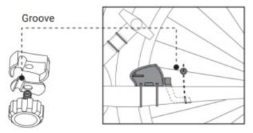
5. Check whether the crank magnet and spoke magnet are aligned with the sensing position of the sensor, and the distance between them should be less than 30mm, and fix the tail of the sensor with screw wrench.(Notice:
