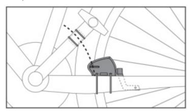
4. Attach the groove of the spoke magnet to the bicycle spoke, align it with the sensing position of the speed sensor, and tighten it. Groove
