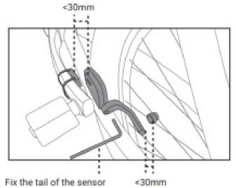
6. Check whether the installation is successful. Turn the crank and the back wheel of the bicycle, speed LED shows blue color, cadence LED shows green color. After confirming that the installation is successful, tighten the cable ties and cut off the excess parts, and fix all the accessories with the rubber band. LED Light
