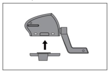
3. Align the sensing position of the cadence sensor with the crank magnet, and install it as the picture shows below, fix it with cable ties.
