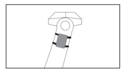
2. Install the rubber pad onto the main sensor.
