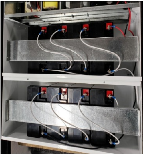
Battery brackets installed on the front
