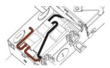
5. Place the Driver Box thru the opening and latch the junction box to the driver box. Mount to structure if required by code.\*
