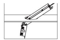
6. Route the low voltage cable to additional downlight locations. Pull enough slack through each hole to make connecting the fixtures easier. Adhere Power Supply Labels (G) at ~10-foot intervals by folding onto the cable then bundle and store the remaining length in the ceiling.
