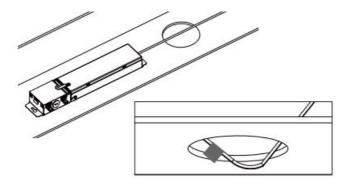
7. Attach the termination cap (F) to the end of the low voltage cable. Use the reusable cable tie to bundle the remaining cable and store it in the ceiling. DO NOT CUT
