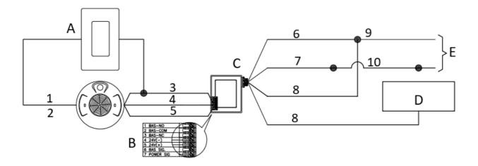
A: GMDS-W B: OCS-L-D-\* C: RSP-V-SW D: LOAD E: LINE
