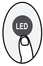
Press this button to turn on and turn off the display on the indoor unit.
