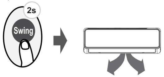
Keep pressing this button more than 2 seconds, the vertical louver swing function is activated (Model dependent) **Airflow direction**
