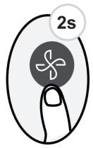
Keep pressing Fan button for more than 2 seconds to activate/disable Silence function(some units) Due to low frequency operation of compressor, it may result in insufficient cooling and heating capacity. Press ON/OFF, Mode, Sleep, Turbo or Clean button while operating will cancel silence function **FP** function
