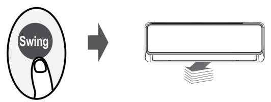
If continue to press the SWING button, five different airflow directions can be set. The louver can be move at a certain range each time you press the button. Press the button until the direction you prefer is reached.
