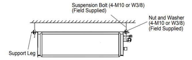
Fig. 4.5 Installation of Indoor Unit
