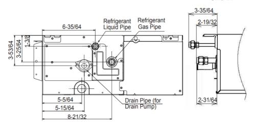
Fig. 5.1 Piping Connection Points
