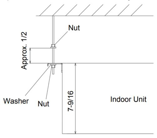
Fig. 4.6 Suspension Bolts and Nuts
