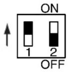
\* Once strong current is accidentally connected to Terminals 1 and 2 of TB2, the PCB fuse will be blown. Then, it's necessary to correct the wiring and then set switch No. 1 to ON.
