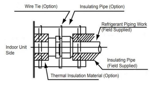
Fig. 5.5 Thermal Insulation of Pipes
