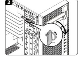
$\bullet$  Install the 3.5  $\!\!\!^{\prime\prime}$  device into the external bay
