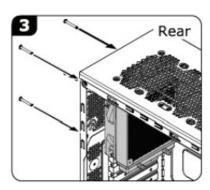
How to install the power supply
