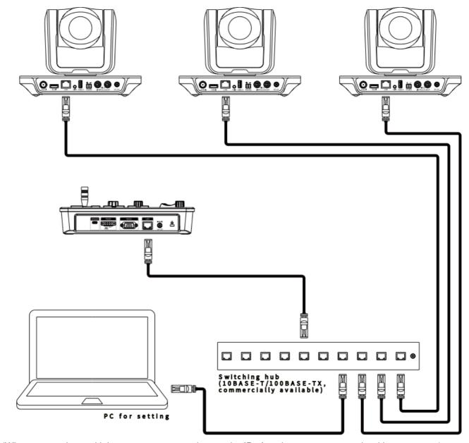
(When connecting multiple cameras, you need to set the IP of each camera separately with a computer).
