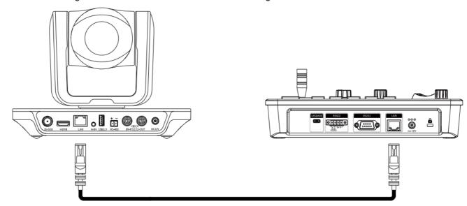
• Connect with multiple cameras by LAN interface detail connection diagram as follows:
