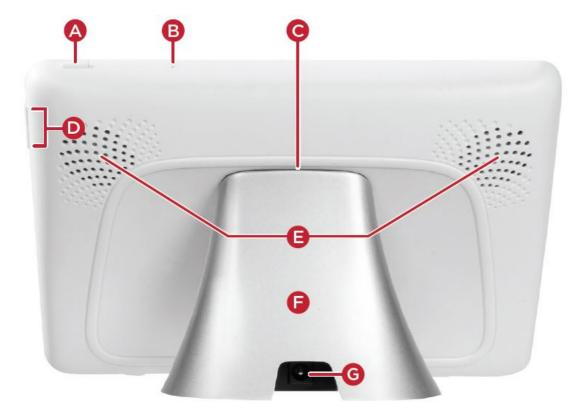
**A** Power button. Press to enter or exit battery saving mode, press and hold to turn off or restart, or press and hold for 10 seconds to power off.
