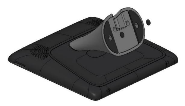
9. Install the threaded posts (all thread) into the base of the charging station.
