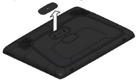
2. Use the Phillips-head flat screws provided in the kit to install the permanent-mount adapter into the touchscreen's docking
