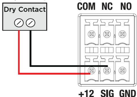
• Wire the contact to an externally powered sensor (Driveway sensor)
