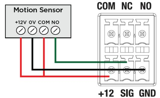
Wire the contact to a dry contact sensor (Door contact sensor)
