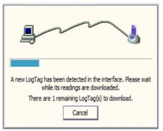
A few seconds later the chart/data will pop-up on the screen and then the following message: Click OK in the box and remove the data logger from the docking station.
