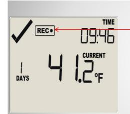
Once READY disappears, immediately release the button. STARTING will also disappear, and the symbol <u>REC•</u> will be shown. The VFC 400 is now recording temperature data.
