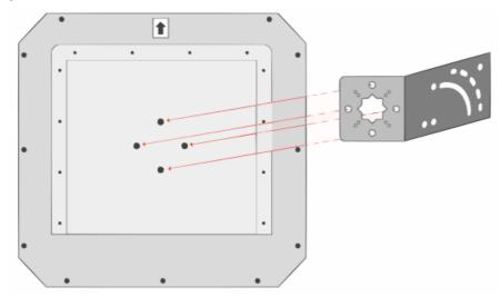
• Use the support piece clamps and fixed wrench to place the iDUHF Lite on the support mast previously installed in the environment.
