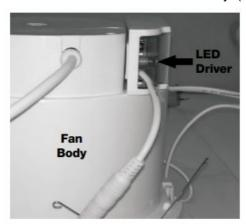
2. Plug the Fan and LED driver into a socket outlet. Knock out the stamped tab in the motor body and feed the LED output connector through. (See diag. 2)
