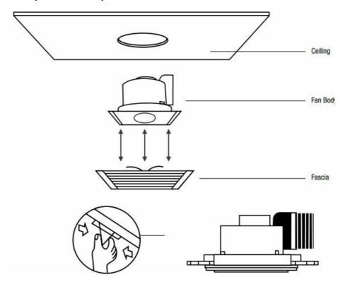
Note: When installing the fan in a bathroom, the duct should decline downwards about 10 degrees
