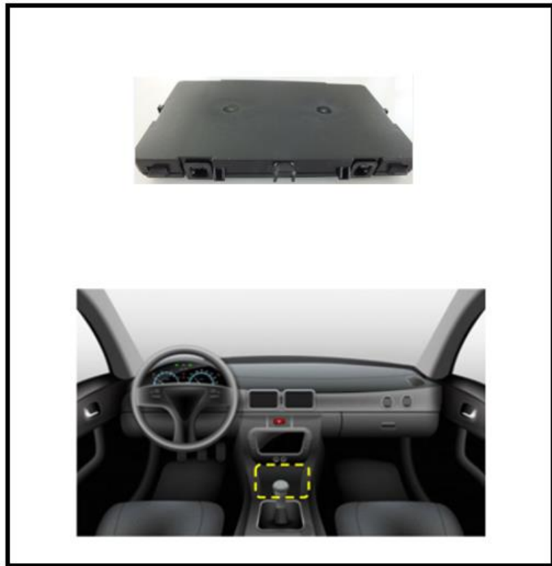
Fig. 1: NFC 3.0 module and its implementation inside the vehicle
