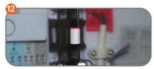
Push out the cut out on the bottom of the cover of the Quant um wiring extension-RF.
