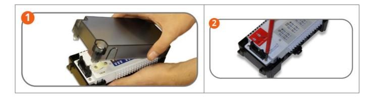
Remove the plastic cover. Open the four white screws with a quarter turn only.
