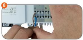
Attach the white strain-relief using the two screws to secure the power wires.
