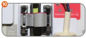
Remove the plastic cover from the Quantum wiring centre-R
