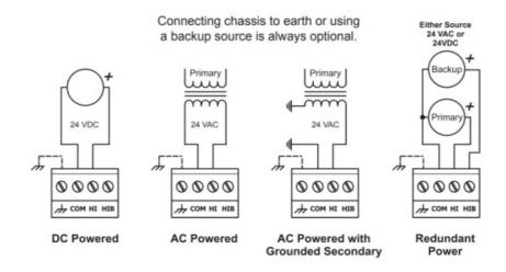
**WARNING:** Internally, this device utilizes a half-wave rectifier and therefore can only share the same AC power source with other half-wave rectified devices. Sharing a common DC power source is also possible. Sharing AC power with full-wave rectified devices is NOT recommended. Devices powered from a common AC
