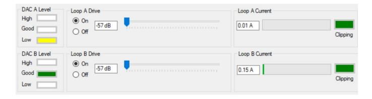
**DAC A/B Level** – Indicates the level of the audio signal being fed to each output channel's DAC. This is the signal level after pre-amp gain, processed by AGC, HPF, HFC, but before any Output drive level has been applied. Make sure to keep it in the "good" range.
