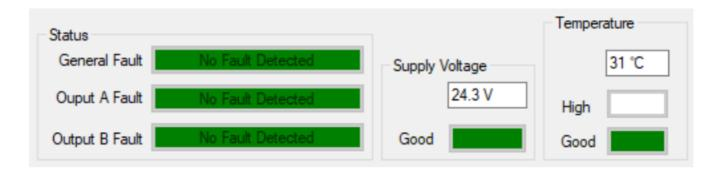
This section displays any potential faults, as well as the internal power supply's voltage and internal temperature. If no faults are detected (as in the image above) all indicate "no fault detected" on a green background. If, however, a fault is detected, the colour changes to red and the fault is presented.
