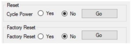
The Reset and Factory Reset section allows the VLD1 to be power cycled or restored to factory settings.
