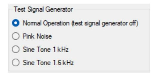
This feature provides the required signals needed for setting up a loop, negating the need for an external signal generator.
