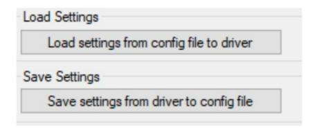
The software can save all settings stored on the driver to a config file. This can then be used to load these settings to the same or another driver without the need to manually change all settings.
