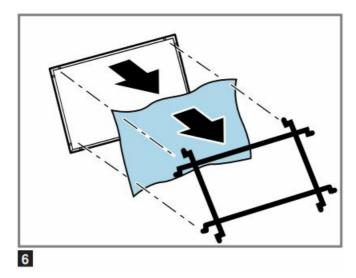
Place the new odor filter onto the rear of the grease filter and use the grid to secure the odor filter to the outer holes. → Fig. 5
