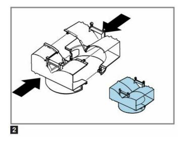
Screw the circulating air guide to the retaining bracket. → Fig. 3
