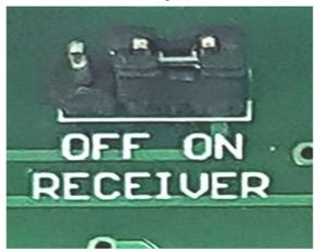
To disable the wireless receiver and use it solely as a soft start, remove the jumper link and place it on the "Receiver-OFF" and middle pin. In this mode, the light will go green momentarily then go to red enabling the output.
