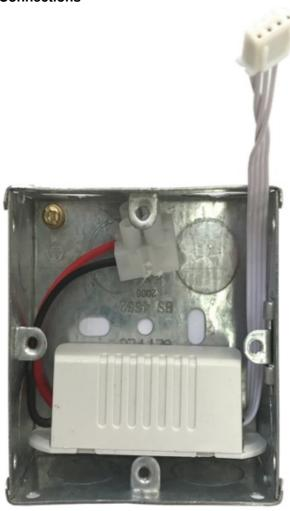
The power supply must installed exactly as per picture, otherwise it will not fit. Line and neutral 230VAC must be connected to the power supply via a 3A fuse.
