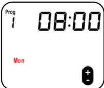
• **Step 6:** Press the PROG button. Prog 1 in the top left of the display should flash. Use the + button to increment this to Prog 2.
