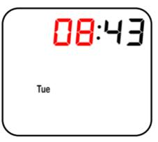
• Step 3: Press the TIME button. The day will flash. Use the + and – but-tons to change the day. Once set, press the TIME button to return to the main screen.
