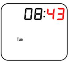
• Step 2: Press the TIME button. The hours will flash. Use the + and – but-tons to adjust the hours.
