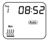
Mode In this mode, the heater will follow the week's time/temperature program. The temperature can be temporarily overridden in AUTO mode by using the + and – buttons to set the new temperature. The new set temperature will be then maintained until the next program step.
