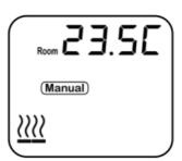
The FAN mode is only available if there is no demand for heating. If the CRXSLWIFI shows heating symbol the FAN mode isn't available. FAN mode only works with compatible heaters.
