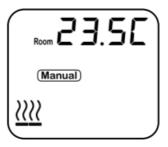
In MANUAL mode, the heater maintains a chosen set temperature between  $4^{\circ}$ C and  $35^{\circ}$ C. To amend the set temperature when in MANUAL mode, use the + and – buttons . Once the temperature is set, you can leave the display to return to the main screen and the settings will be saved. When the room temperature reaches the set temperature, the heating will be deactivated.
