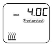
In FROST PROTECT mode, the heater maintains a chosen set temperature between 4°C and 15°C. To amend the set temperature when in FROST PROTECT mode, use the + and – buttons. Once the temperature is set, you can leave the display to return to the main screen and the settings will be saved.
