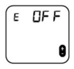
If this is **ON** the back light will be permanently on when the heater is active.
