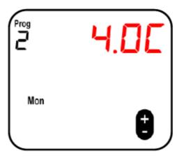
• Step 9: Repeat these steps for programs 3-6 if additional time periods are required. Any programs not being utilized must be deactivated. To do this, simply select the program in question as per step 6 and press the STANDBY button.
