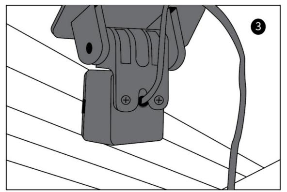
Flip down the leveler at the rear of the sensor and adjust the bracket until the bubble in the leveler is located within the center of the two vertical black lines, then tighten the knob.
