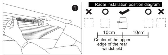
Find a position ±10cm at the center of the upper edge of the rear windshield with a tape measure, and wipe it with an alcohol pad/ clean rag.
