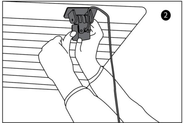
Tear off the tape of the bracket of the sensor, and attach the base bracket parallel to the ceiling. It is recommended to attach the device close to the ceiling or align along the defog line. Be careful not to attach it to the defog line. Or stick on the top side of the rear windshield, like the below picture shown.
