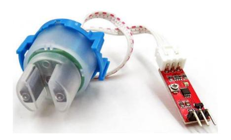
The Water Turbidity Test Sensor for Arduino is a sensor designed to measure the turbidity of water. It can be connected to an Arduino board and used to monitor the clarity of water in various applications.
