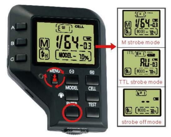
Press (MENU] button to switch the strobe modes Select the desired mode, and press (ENTER] to confirm
