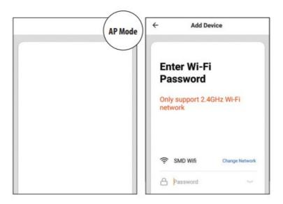
In the Connex Connect App top right corner of the device screen, click "+". Select "AP Mode" in top corner. Select "next" and enter your Wi-Fi and password details.
