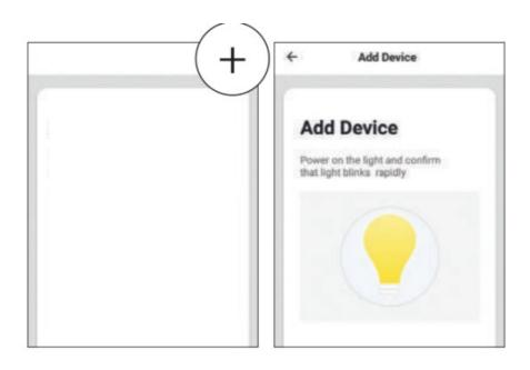
In the Connex Connect App top right corner of the device screen, click "+". Make sure the bulb is flashing rapidly indicating "ready to connect".
