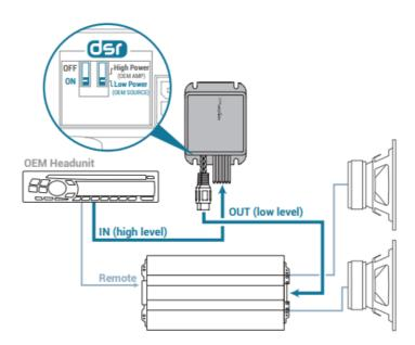
**DSR:** DOUBLE STEP-DOWN RATIO, allows correct level interfacing with OEM Headunit or OEM Amplifier by switch selection.
