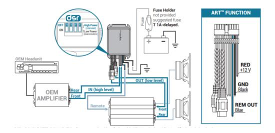
**DSR:** DOUBLE STEP-DOWN RATIO, allows correct level interfacing with OEM Headunit or OEM Amplifier by switch selection.
