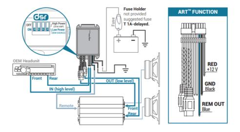
**DSR:** DOUBLE STEP-DOWN RATIO, allows correct level interfacing with OEM Headunit or OEM Amplifier by switch selection.
