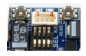
Notes To activate any of the features, momentarily connect the signal the GND provided on the connector using momentary close switches only.
