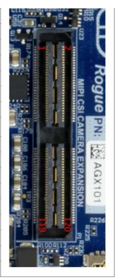
Only 6 of the CSI2 interfaces can be used at once in 2 lane configuration. Only 4 interfaces when u sing 4 lane configuration.
