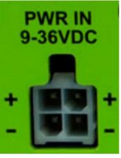
**Note:** A Power Supply capable of 100W or more is required to operate the Rudi-NX with all peripherals running at their respective maximum rating.
