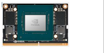
**Note:** A Thermal Transfer Plate is mounted to the NVIDIA Jetson Xavier NX module internally to the Rudi-NX. Heat will dissipate through to the top of the Rudi-NX chassis.
