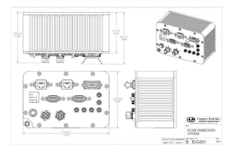
ISO View - Rosie Embedded System with Mounting Brackets
