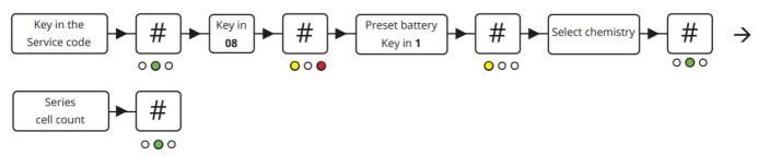
Here is an example of how you preset the battery when having a 12V Lead Acid with 6 cells. See following instructions.
