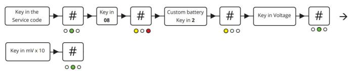
Here is an example of how you preset the customized battery low warning. In this example we want the battery to send a warning at 10,8V.
