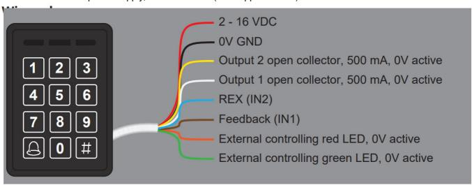
**Note:** Right after applying the voltage all LED's lights and the buzzer sounds **do not** touch the reader until the yellow LED lights and the buzzer is silent.
