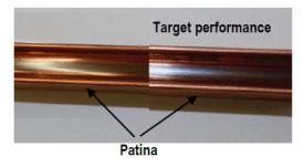
• Cleaned copper rail (copper coloured rail with scrub marks)
