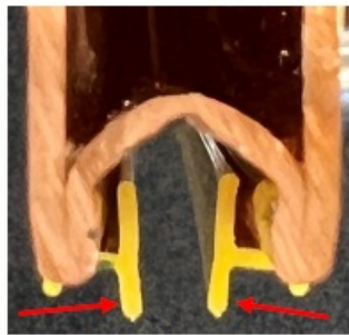
Fig. 19: Distortion of the insulating profile inner bar
