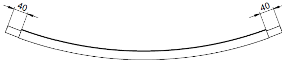
Fig. 26: Inner bend with centrally aligned insulating profile
