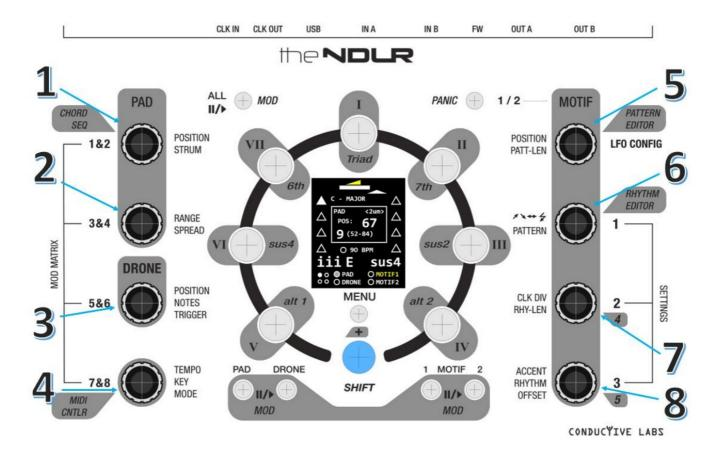
**a.** The 8 knobs labeled 1 through 8 are also buttons. From the home screen, press the knobs to change the parameter the knob controls, as labeled on the inside of the knobs. The Triangle in the window will rotate to indicate the current parameter. Some knobs have 2 choices, some have 3.
