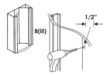
2. Insert elephant anchors by folding metal channel until it is flat with the plastic straps. Slide the metal channel into the drilled hole.
