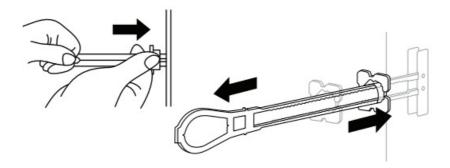
5. Place thumb between plastic straps. Push side to side, snapping off straps at wall.
