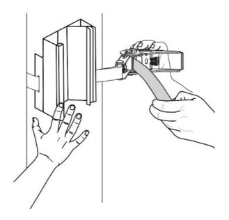
Crank the handle to tighten the strap until it feels taut and secure.
