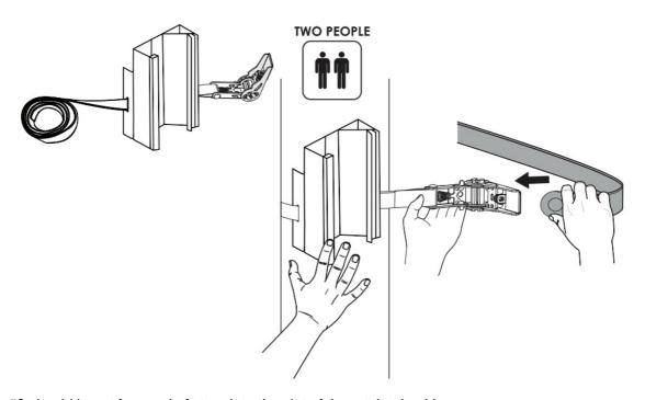
5. Person #2 should insert free end of strap into the slot of the ratchet buckle
