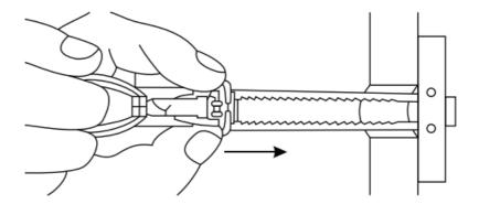
4. Hold ends of straps together between thumb & four finger and pull toward you until channel rests behind wall.
