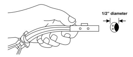
3. Hold the plastic straps by the end and pull towards you until the metal channel is flush behind the wall.
