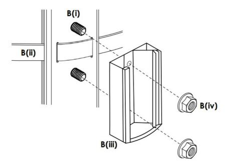
3. Hold column mounting bracket to the column where you would like to mount the shelve
