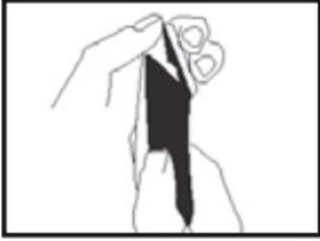
To remove blade set from your trimmer, make sure the trimmer is in the OFF position. Remove the blade set by placing thumb against the smaller cutter and pushing forward, releasing the cutter assembly from the trimmer housing. Replace with new cutting system and reverse the removal procedure, only this time place your thumb on the large cutter and snap into place.
