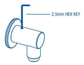
3. Ease the Wall Outlet Elbow off the spigot ensuring the grub screw does not come into contact with the o-ring seal.
