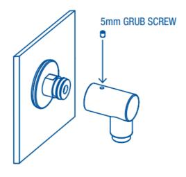
4. Once exposed, unscrew the spigot from the thread using a spanner.
