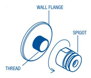
5. Once spigot has been removed from thread, use a hand tool to lever circlip from spigot and remove flow control.
