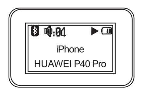
**Note:** The default play source is the first connected device. If you want to switch the playback device, please hit pause on the current device, then hit play on the other device.
