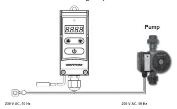
**Warning!** Always take into account the load ability of the controller relay when connecting (10 A (3 Inductive load)) and follow the instructions of the manufacturer of the pump which you would like to control.
