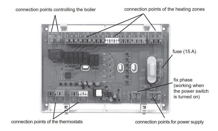
In case of using electro-thermal zone valves that operate slowly and all the zones are closed when the boiler is inactive, then the boiler should be started with a delay in order to protect the pump of the boiler. In case of using electrothermal zone valves that operate fast and all the zones are closed whenthe boiler is inactive, then the valves should close with a delay in order to protect the pump of the boiler. See Section 5 for more information on the delay funcions.
