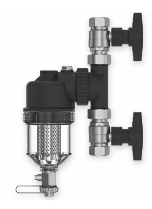
Contaminants are always present in heating and cooling systems. They can accumulate over time and can cause clogging, failure, performance degradation, or noise. To prevent this, dirt must be separated from the system. The COMPUTHERM DS5-20 and DS5-25 magnetic dirt separators serve this purpose, with their design, filter and strong magnet, they effectively remove both magnetic and non-magnetic dirt from the heating/cooling systems, allowing the
