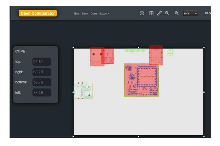
Here is nicely arranged small board with previously selected functions:
