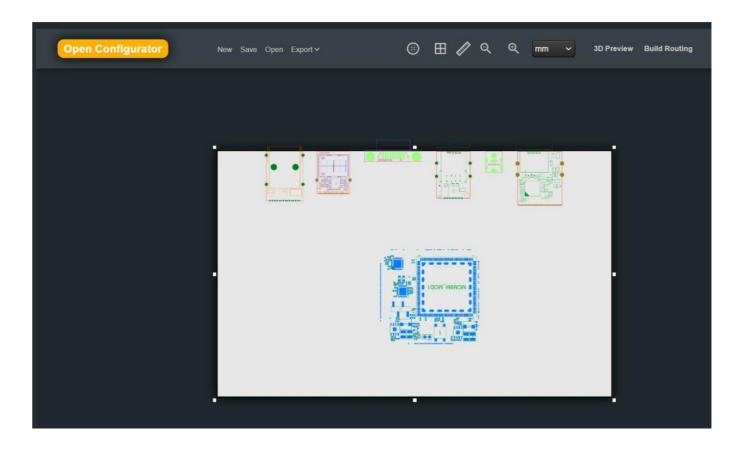
Now you can resize the board as you wish and drag peripheral functions to the required positions.
